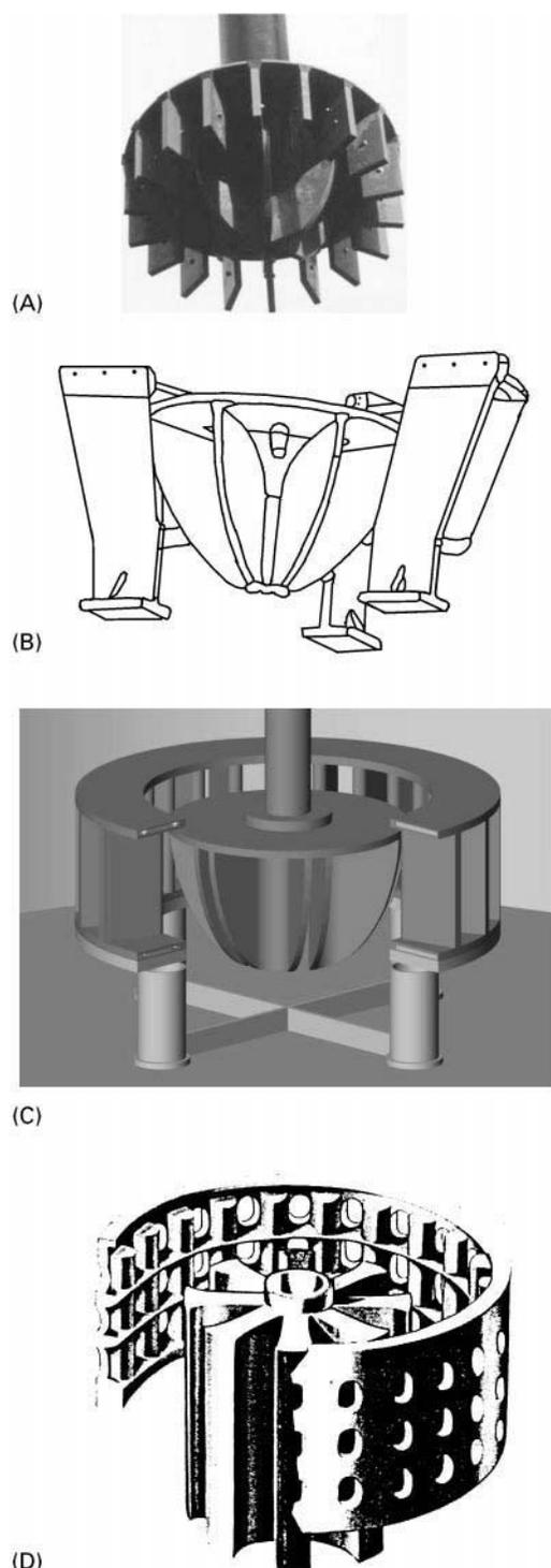
**Figure 7** Shapes of different impellers and stators. (A) Bateman; (B) Dorr-Oliver; (C) Outokumpu; (D) Wemco (courtesy of Bateman Process Equipment, Dorr-Oliver, Outokumpu Mintec Oy and Baker Process, respectively).
