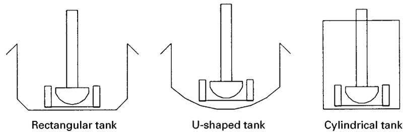
**Figure 5** Typical tank designs in mechanical flotation cells.
