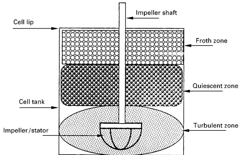
**Figure 2** Hydrodynamic zones in a mechanical flotation cell.
