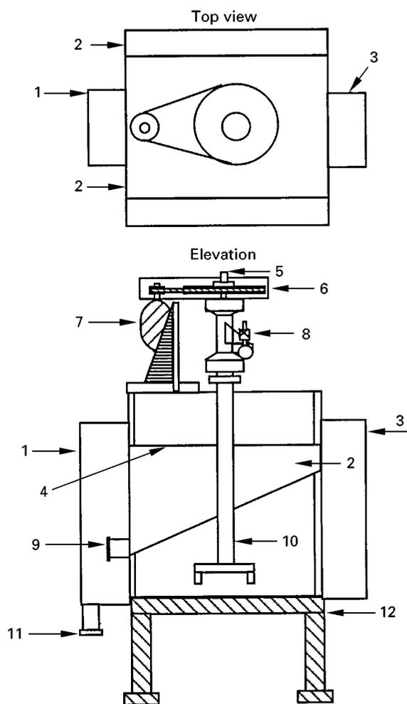
**Figure 1** Schematic diagram of a mechanical flotation cell. 1, Discharge box; 2, concentrate launders; 3, feed box; 4, cell lip; 5, bearing shaft; 6, drive pulley with guard; 7, three-phase induction motor; 8, air inlet pipe with control valve; 9, concentrate launder discharge point; 10, impeller shaft; 11, tailings discharge point; 12, base support for the cell tank.
